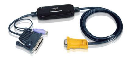
CV130A is a signal converter specifically designed for SUN systems. They can be used with KVM switches. Both models have SUN-supported built-in 13W-3 video out and Mini Din-8 keyboard and mouse ports.
