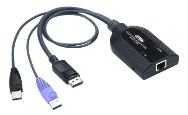
The KA7189 KVM Adapter Cable connects a KVM switch to the DisplayPort video and USB ports of a target computer.\* The KA7189 supports DisplayPort output and provides two USB plugs to connect a target computer for keyboard/mouse, Virtual Media, or Smart Card/CAC Reader functions.\*\*
