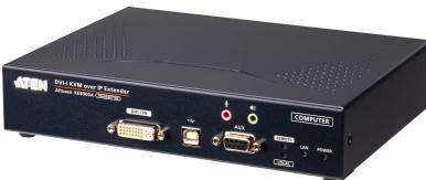
The KE6900A extenders are consisted of a high performance IP-based transmitter (KE6900AT) that connects to the computer. The KE6900A allows extended access of computer systems remotely via USB consoles (USB keyboard, USB mouse, DVI monitor) over intranet, enabling users to place the computer system in secure and temperature controlled environments, which maybe isolated from users' workstation.
