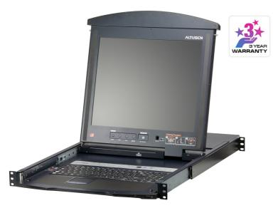
ATEN KL1508A LCD KVM Switch features independently retractable, dual slide 17" or 19" LED-backlit LCD monitor and keyboard with built-in touchpad. The KL1508A KVM switches are control units that allow IT administrators to access and control multiple computers from the LCD console and an extra PS/2 or USB KVM console.
