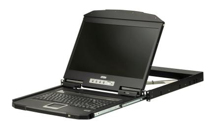
The CL3700 USB HDMI LCD Console is a short depth single rail LCD KVM console featuring an 18.5" LED-backlit widescreen LCD monitor with an integrated keyboard and touchpad. The short-depth design fits all 19" equipment cabinets, and is especially suitable for shallow racks. The CL3700 provides an ideal space-saving solution for special environments such as outside broadcast vans (OB vans) and compact control rooms.
