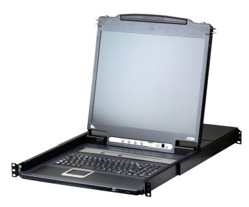
The CL5716I Slideaway<sup>TM</sup> LCD KVM Switch is a control unit that allows access to multiple computers from a single PS/2 or USB KVM (keyboard, video, and mouse) console. A single CL5716I can control up to 16 computers. Up to 15 additional KVM switches can be daisy-chained to the CL5716I, so that up to 256 computers can all be controlled from a single KVM console.
