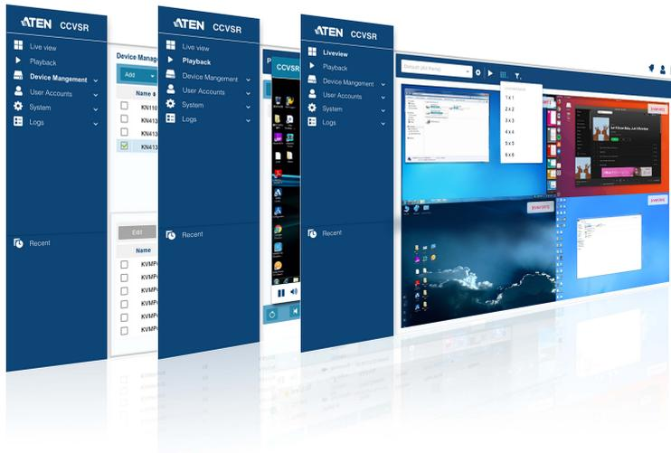
ATEN's Control Center Video Session Recording (CCVSR) software is an innovative and effective solution designed for live monitoring and operation backtracking. Administrators can view live feed of operators currently operating on their systems and thus quickly resolve operational flaws, process discrepancies, etc. On the other hand, IT managers can go back to recorded operation videos to trace changes made for compliance control improvement and auditing efficiency.
