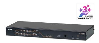
The KH2516A KVM switch is a control unit that allows IT administrators to access and control multiple computers from two PS/2 or USB KVM consoles (one bus). Operators working at up to two consoles can independently and simultaneously take control of up to 16 computers. By daisy chaining up to 15 additional switches, as many as 256 computers can be controlled from the original KVM consoles
