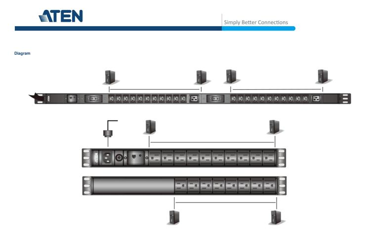
Note: (1) As there are many Basic PDUs, PE0324S (top) and PE0118S (bottom) are the respective 0U and 1U examples used here.
