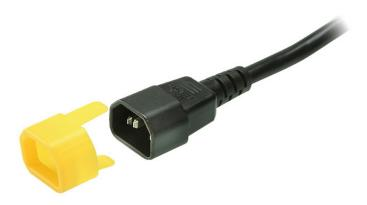
For better power stability, ATEN has developed the EZ-Lok Plug Connector to secure the connection of a power cord's plug with the PDU outlet. With a simple installation, the EZ-Lok Plug Connector will ensure that the power cord and PDU outlet never come apart without your assistance.
