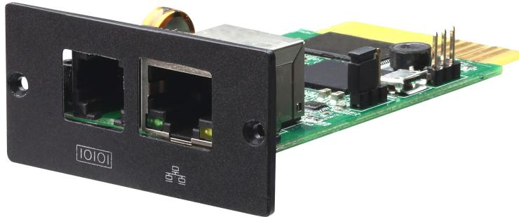
ATEN's SP100 (SNMP card) is an UPS monitoring equipment. Allows connection of the UPS directly to the ethernet network through a RJ-45 connector without using RS-232 ports on the computer and without loading any individual UPS management software on the network server. User can remotely control the UPS and monitor UPS current status from any off site location. SP100 can communicate the status of a UPS and issue commands to it.
