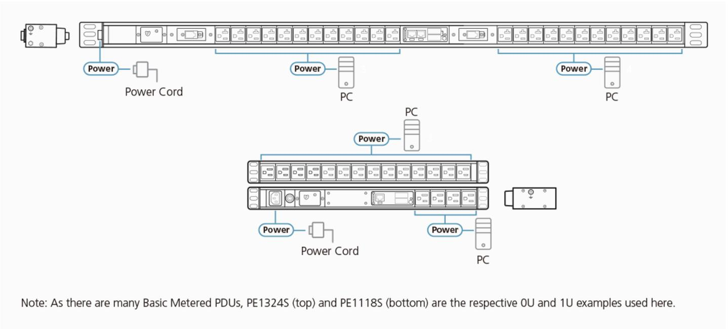
Note: As there are many Basic Metered PDUs, PE1324S (top) and PE1118S (bottom) are the respective 0U and 1U examples used here.
