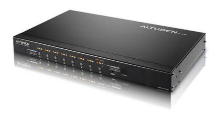
The PN9108 Power over the NET™ is a control unit that provides remote power management for eight AC outlets via a TCP/IP connection, allowing administrators to control the power off, power on, and reboot status for each attached device from any computer connected to the Internet, whether down the hall, or half way around the world. The PN9108 is the most convenient, reliable and cost effective way to obtain access to your server room remotely.
