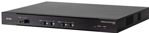
AP412 is a 4-channel DSP-equipped amplifier that delivers 120W per channel and receives balanced / unbalanced mic / line-level signals to drive 4 / 8-ohm low impedance or 70 / 100V line loudspeaker systems. It also supports Lo-Z / Hi-Z in Bridge mode to deliver higher power.
