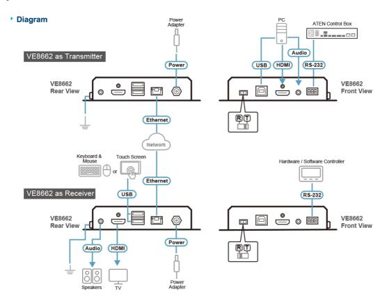
Note: The illustrated diagram is based on two VE8662 units.
