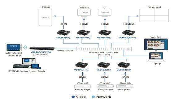
Note: VE8662 supports PoE and can be installed in combination with PoE network switches to reduce power cabling and additional power outlets. Before choosing the Network switch and installation, please refer to the Implementation Guide.
