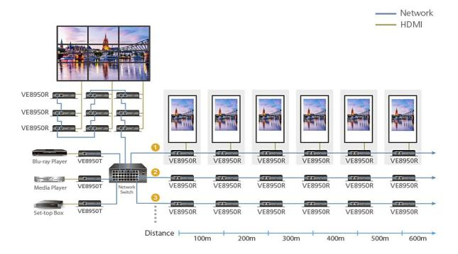
\*Use daisy chains to configure a video wall or expand the AV system hundreds of meters
