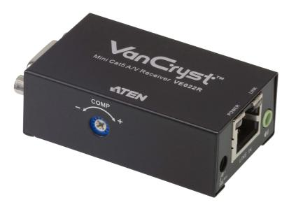
The VE022R Mini Cat 5 A/V Receiver connects with a <u>VE022</u>T to extend signals up to 150m from the source using a Cat 5e cable. With hot-plugging support, you can quickly add or remove the VE022R receiver connected to the display device without having to power down any of the devices. The <u>VE022</u> Mini Cat 5 A/V Extender is a compact, convenient and economical addition to your video/audio setup.
