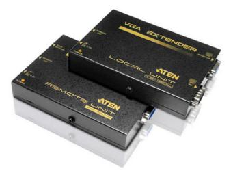
VE150 video extender comprises a local transmitting unit and a remote receiving unit which are connected by standard Cat 5e cables. The distance of both units can be extended up to 500 feet (150m). It is ideal for factories and construction sites, or any location where the display may need to expose in a risky setting, but you want the system to be kept in a safe location.
