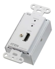
ATEN VE1801UST is a transmitter designed to reliably send 4K signals up to 40 m over a single Cat 5e/6/6a or ATEN <u>2L-2910</u> Cat 6 cable. With US Wall Plate design, the VE1801UST can be conveniently mounted in a one-gang junction box. For HDMI signal transmission, it supports 3D, Deep Color, and embedded HD lossless audio formats.
