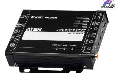
The VE2812R is a high-quality HDMI HDBaseT Receiver featuring audio de-embedding function. Powered by HDBaseT™ technology, the VE2812R can receive 4K HDMI signals up to 100 m over a single Cat 5e/6/6a or ATEN 21-2910 Cat 6 cable. With HDBaseT Long Reach Mode enabled, it can deliver HDMI signals up to a maximum range of 150 meters @ 1080p.
