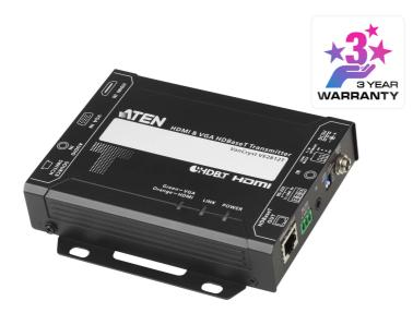
ATEN VE2812T is a transmitter for sending VGA (with audio) and HDMI signals up to 100 m over a single Cat 5e/6/6a or ATEN <u>2L-2910</u> Cat 6 cable. The VE2812T guarantees reliable transmission of HDMI signals, supporting 3D, Deep Color, and embedded HD lossless audio formats. It also ensures transmission of VGA (with audio) at distance up to 100 m. In addition, it supports Long Reach Mode up to 150 m via a single Cat 5e/6 cable at resolutions up to 1080p.
