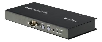
The <u>VE500R</u> is the Cat5 Audio / Video a receiver, part of an ATEN A / V extension solution. The unit is designed to integrate into installations with ATEN's <u>VM0808T</u> A / V matrix switch. It can also be used in conjunction with a <u>VE500T</u> transmitter as a point to point stand alone A / V extender to a maximum distance of 500 ft.
