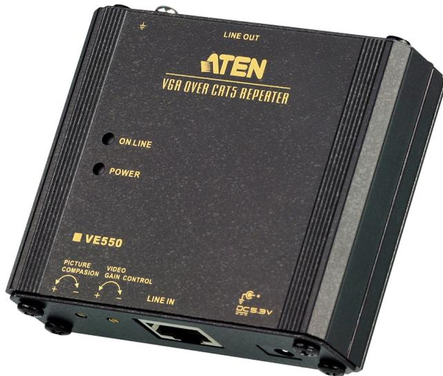
The VE550 VGA Over Cat 5 Repeater is a video signal extension device which is compatible with ATEN KVM Extenders, Video Extenders, and Cat 5 KVM Switches. The VE550 extends the video transmission range up to twice the original distance over Cat 5e cables. Moreover, using an additional repeater, VGA signals can be transmitted over even longer distances.
