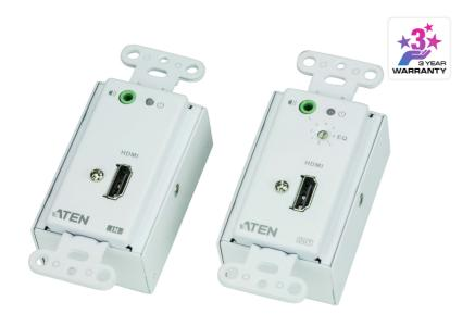
The VE806 HDMI Over Cat 5 Extender Wall Plate extends HDMI and audio signals up to 200 feet (60m) using Cat 5e cable. It supports popular wide screen formats and ensures excellent video quality over long distance transmissions. The VE806 combination can further extend the distance or multiply sources/displays.
