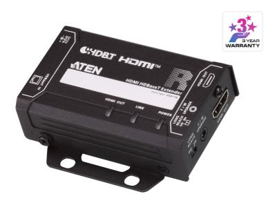
The ATEN VE811R HDMI HDBaseT Extender guarantees the optimum 4K HDMI signal transmission across up to100 m via a single Cat 5e/6/6a or ATEN 2L-2910 Cat 6 cable. In addition, with the support for Long Reach Mode, it extends HDMI signals @ 1080p up to 150 m via a single Cat 5e/6 cable. The VE811R meets HDMI specification features including 3D, Deep Color, HD lossless audio formats and CEC pass-through. Plus, it supports Dolby Digital 5.1 and DTS HD audio.
