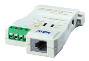
IC485SN is a 2-way converter for converting RS-232 signals to and from RS-422/RS-485 signals in long-distance applications up to 1200 m (4000 ft.) – without the need of an external power supply.
