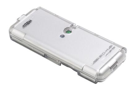
UH275 is a hub with 4 built-in USB2.0 ports. It has LEDs to indicate the connections status, and its handy and slim design allows users to carry it in pockets.
