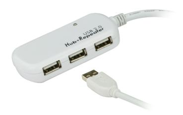
The UE2120H allows users to extend the distance between a computer and USB device(s) up to 40 feet (12 m) via the active extender hub. USB signals transmitted through these cables maintain optimal signal integrity and meet USB 2.0 standards. Up to 4 extender cables (<u>UE2120</u>) and 1 Extender Hub (UE2120H) can be chained together, so that cable distance is increased by up to 200 feet (60 m).
