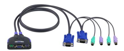
CS62 2-port KVM Switch has a handy design integrating with 1.2m of cable. It can control 2 servers via a single console.
