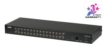
The KH1532A KVM switches are control units that allow IT administrators to access and control multiple computers from a single PS/2 or USB KVM console (keyboard, monitor, and mouse). Operators can take control of up to 32 (KH1532A) computers. By daisy chaining up to 31 additional switches, as many as 1024 computers can be controlled from a central KVM console.
