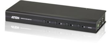
The CS74D 4-Port USB DVI KVM Switch allows you to control four computers using one USB mouse, USB keyboard and Digital Visual Interface (DVI) monitor console. It supports digital video devices, such as fl at panel displays, data projectors, plasma displays and digital TVs.
