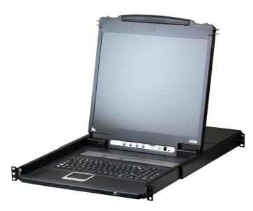
The CL5708I Slideaway™ LCD KVM Switch is a control unit that allows access to multiple computers from a single PS/2 or USB KVM (keyboard, video, and mouse) console. A single CL5708I can control up to 8 computers. Up to 15 additional KVM switches can be daisy-chained to the CL5708I, so that up to 128 computers can all be controlled from a single KVM console.
