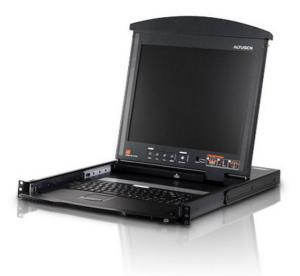
The KL1100 is a LCD KVM console featuring an integrated 17" or 19" LCD panel, a full keyboard, and a touch pad in a 1U rack-mountable sliding housing with AC or DC based input power sources. For added convenience, ports for an external PS/2 or USB keyboard and mouse as well as a monitor are provided on the rear panel - permitting you to manage the switch from a local console.
