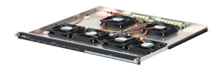
Overheating slows down device performance significantly and can result in equipment breaking down mid-operation. The <a href="M3200"><u>VM3200</u></a> is equipped with a fan module that ensures a cooling system is in place to keep the device from overheating. The fan is hot-pluggable and can be easily replaced without shutting down the system. ATEN ensures that your investment is protected while delivering outstanding performance.
