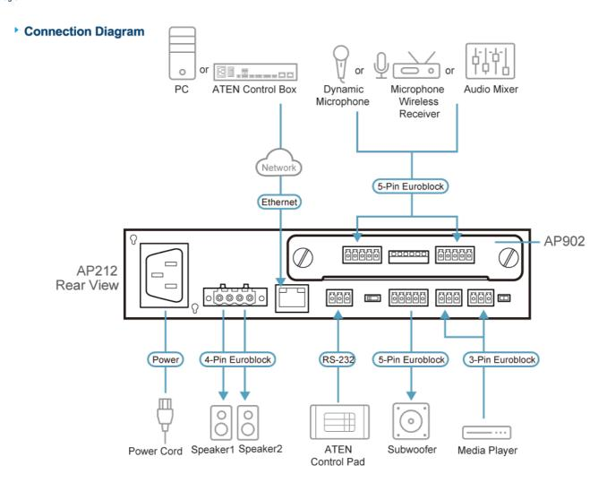
Note: It is strongly recommended that you use a shielded Cat 5e cable (or higher) for better network connectivity.
