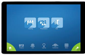
The ATEN VK320 is an 8" Touch Panel featuring capacitive multi-touch IPS-LCD screen with a narrow bezel. Natively installed with the ATEN Control System app, the touch panel is compatible with ATEN Control Boxes and Control Pads.
