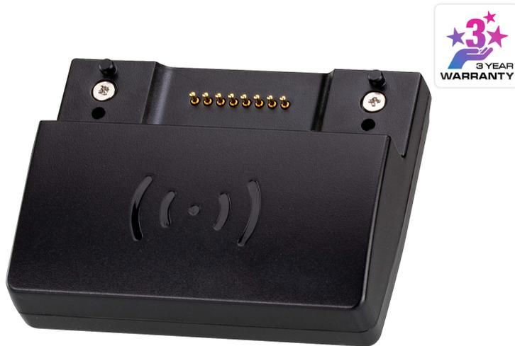
As an add-on accessory designed to complement ATEN's touch panel series ([VK430](#) 10.1" RBS Panel and [VK330](#) 10.1" Touch Panel), the VK401 Access Inspector enhances security and prevents unauthorized usage for credential-based applications. Operating at a frequency 13.56 MHz, this compact access control unit supports multiple standards such as ISO 14443A/B and ISO 15693 and reads smart cards including Mifare and Felica.
