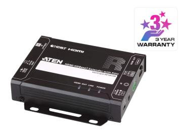
The VE1812R features Power over HDBaseT (PoH) which sends power from Tx to Rx over Cat 5e / 6 / 6a cable without any additional power supply. The VE1812R supports RS-232 and IR signaling pass-through, allowing users to control the HDMI source device from the receiver unit (VE1812R) while also accessing the HDMI display device from the transmitter unit (VE1812T). The IR signals can also be extended in both directions.
