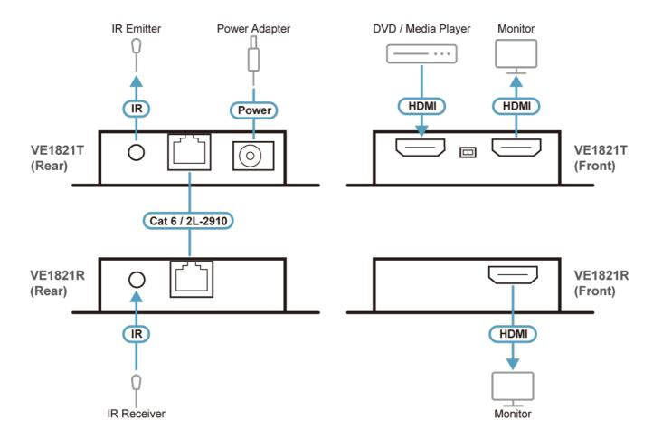
Only connect VE1821T with VE1821R. Connecting VE1821T with other receiver models or third-party receivers may cause physical damage to the receiver.
