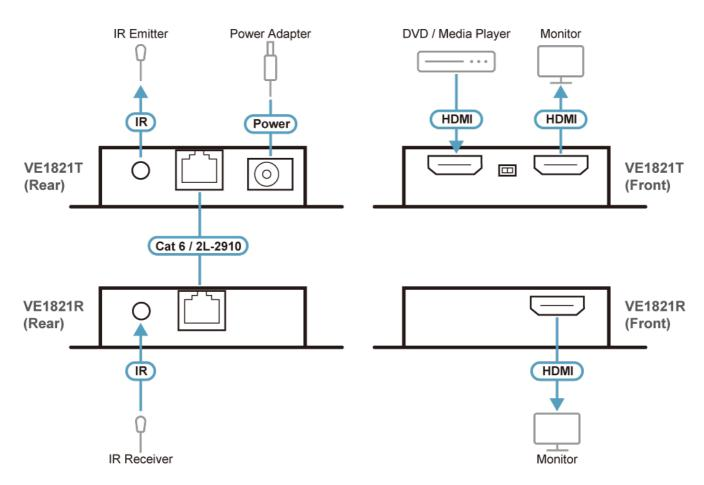
Only connect VE1821T with VE1821R. Connecting VE1821T with other receiver models or third-party receivers may cause physical damage to the receiver.
