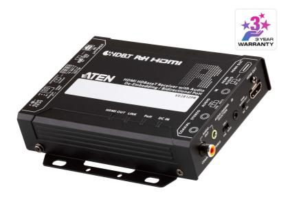
Featuring powerful Class A HDBaseT technology, the VE2812PR is a receiver for 4K HDMI video, audio, and control signals over a distance of up to 100 m via a Cat 5e / 6 / 6a or ATEN 2L-29330 Cat 6 cable. HDMI signal transmission extends further up to 150 m @ 1080p when the HDBaseT Long Reach Mode is enabled.
