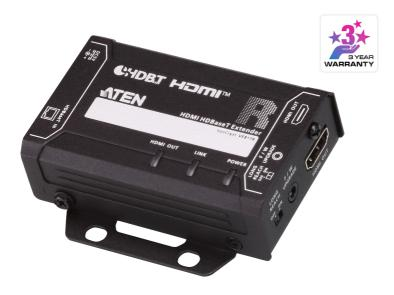
The ATEN VE811R HDMI HDBaseT Extender guarantees the optimum 4K HDMI signal transmission across up to100 m via a single Cat 5e/6/6a or ATEN 2L-2910 Cat 6 cable. In addition, with the support for Long Reach Mode, it extends HDMI signals @ 1080p up to 150 m via a single Cat 5e/6 cable. The VE811R meets HDMI specification features including 3D, Deep Color, HD lossless audio formats and CEC pass-through. Plus, it supports Dolby Digital 7.1 ch and DTS HD audio.
