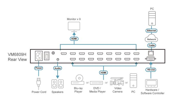
Note: Connects up to 9 display devices to the HDMI output ports, and up to 8 video source devices to the HDMI input ports.
