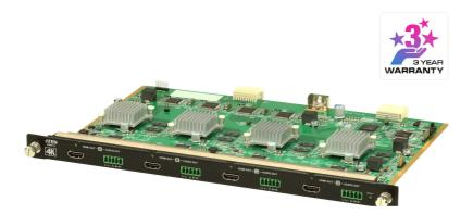
The VM8814 is a 4K HDMI output board that works with an ATEN Modular Matrix Switch to offer an easy way to route 4 HDMI sources to 4 displays. In addition to the HDMI interface that carries digital A/V signals, the VM8814 is equipped with 4 stereo audio output ports that allow HDMI audio extraction.
