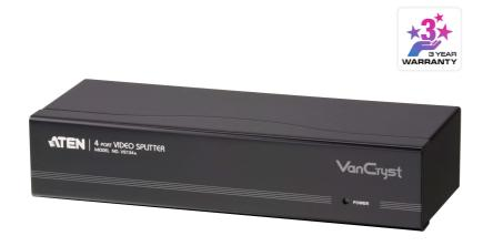
The VS134A Video Splitter is a boosting device that duplicates a video signal from one source to 4 output devices. Cascadable to three levels, the VS134A provides up to 64 video signals, in addition to extending transmission distance up to 30 m, making it excellent for public broadcast systems. To transmit multiple, high-quality VGA, XGA, SVGA, UXGA, QXGA, WUXGA and multisync video signals over long distance without hassle, the VS134A is your best choice.
