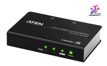
The VS182B True 4K HDMI Splitter is the perfect solution for anyone who needs to send one source of digital high definition video to two displays at the same time. It supports all HDMIenabled equipment, such as DVD players, satellite set- top boxes and all HDMI monitors, displays, projectors, or TVs.
