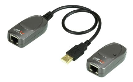
UCE260 can easily send the USB signals via Ethernet Cable up to 60 meters (196 ft) at data rate of High Speed (480Mb/s), Full Speed (12Mb/s) and Low Speed (1.5Mb/s). Without any configuration or software driver, this USB extender allows you to extend your USB device or hub up to 60m from your computer, which overcomes the typical USB cable limitation.
